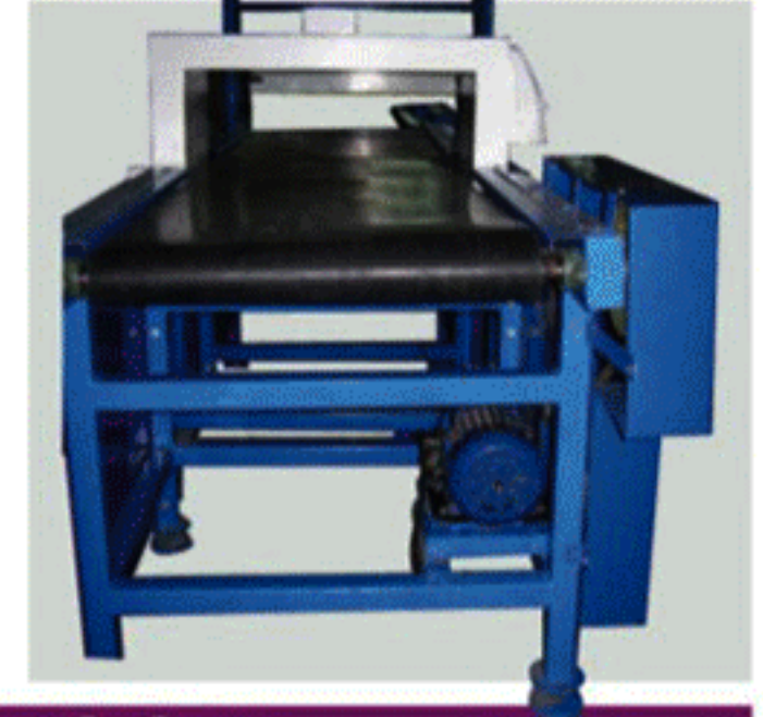
De-magnetizer With Conveyor System
